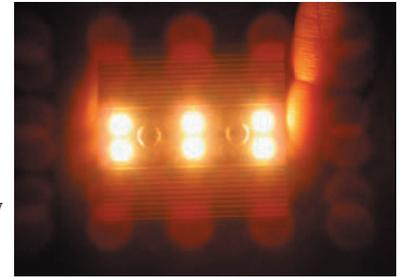
brightness even well below 11 volts. This ability, coupled with its smaller current draw, makes it excellent choice on small boats where lighting is challenged by limited battery capacity.
